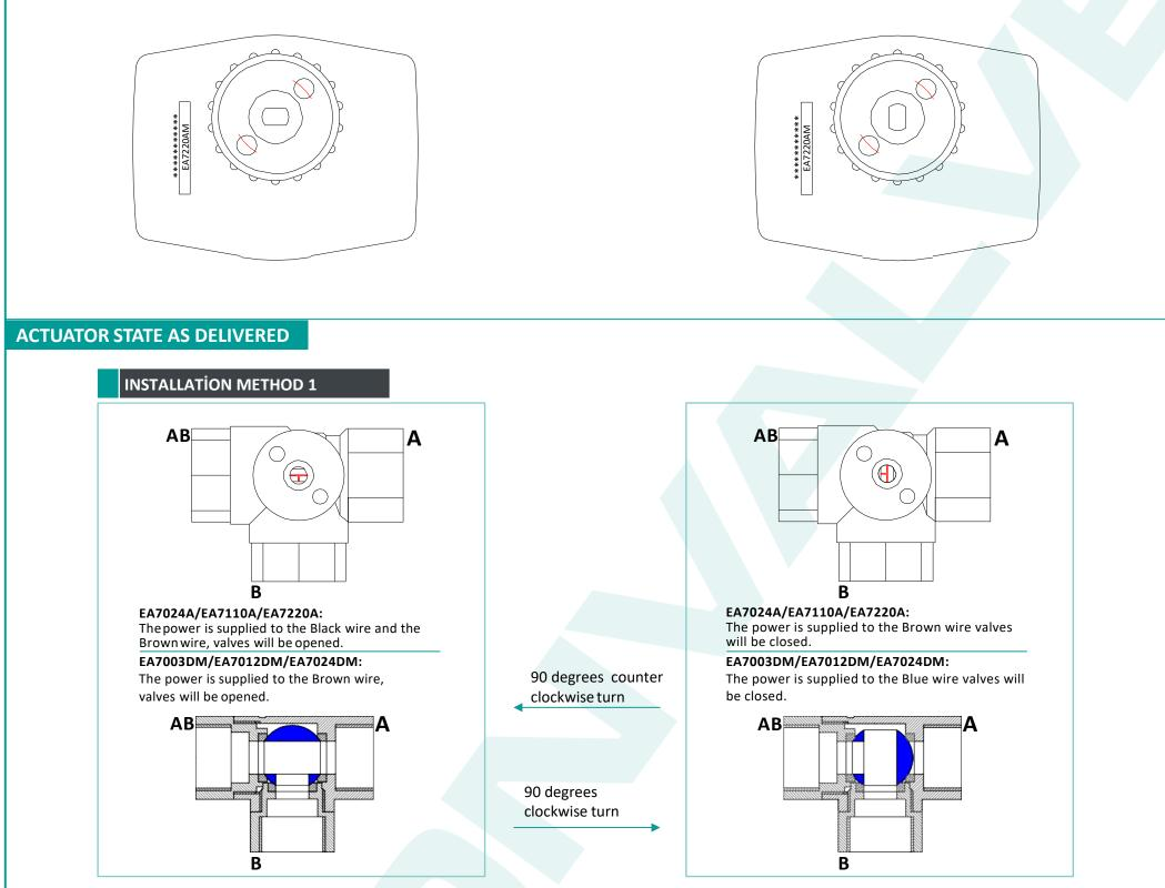
EA7220AM(A)+CBBVM315/20/25. at 90 degrees clockwise and counterclockwise turn. Core Ball is "T" mode.
