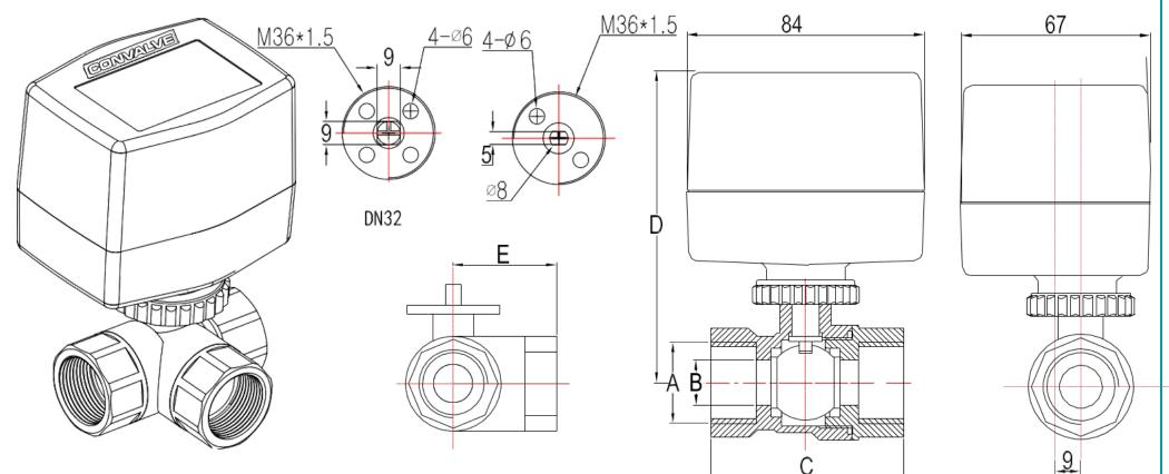
Unit: mm (Allowable tolerance±2)
