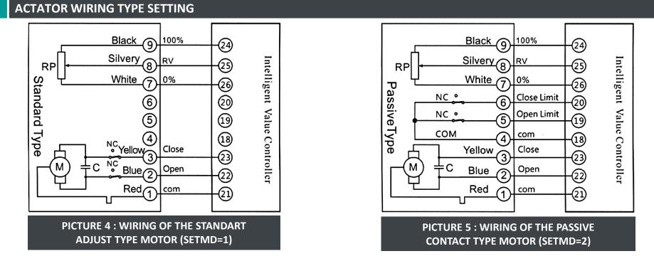
By change P to 9.5, and press "A/M" key to enter Md parameter setting, set the motor type refer to below table.
