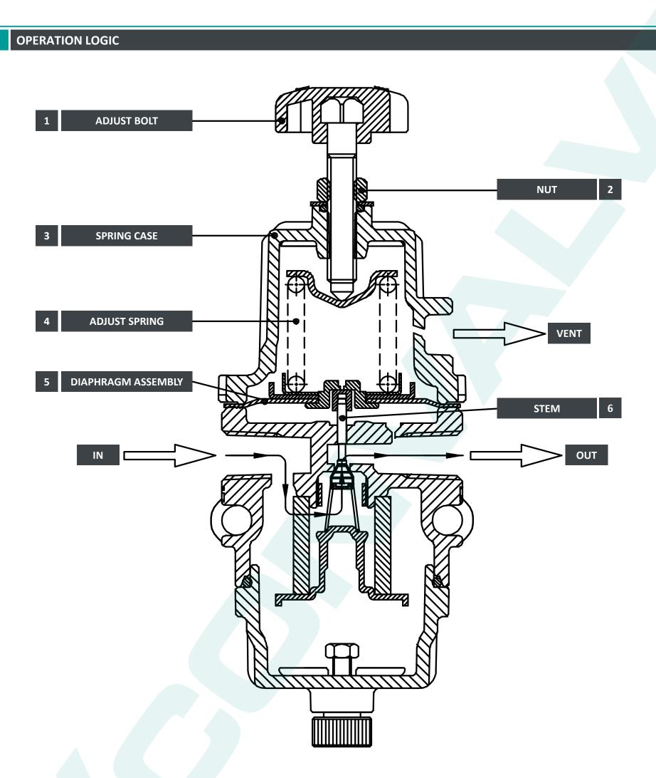
When the adjustment bolt ① is turned clockwise, the adjusting spring ④ exerts force on the diaphragm ⑤, causing the stem ⑥ to move downward. As a result, the supply pressure (IN) is directed to the secondary output port (OUT). As the pressure on the secondary port reaches the set pressure, this pressure is transmitted to the bottom of the diaphragm through the output pressure sensing hole, and the set pressure is maintained by balancing the force with the adjusting spring ④.
